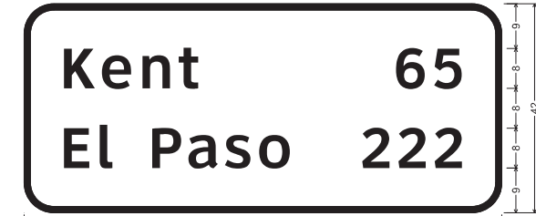
E7-2T_VARx42: 6.0" Radius, 1.3" Border, White on Green; "Kent", ClearviewHwy-5-W-R; "65", ClearviewHwy-5-W-R; "El Paso", ClearviewHwy-5-W-R; "222", ClearviewHwy-5-W-R;
