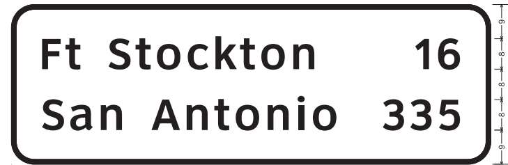
E7-2T_VARx42: 6.0" Radius, 1.3" Border, White on Green; "Ft Stockton", ClearviewHwy-5-W-R; "16", ClearviewHwy-5-W-R; "San Antonio", ClearviewHwy-5-W-R; "335", ClearviewHwy-5-W-R;
