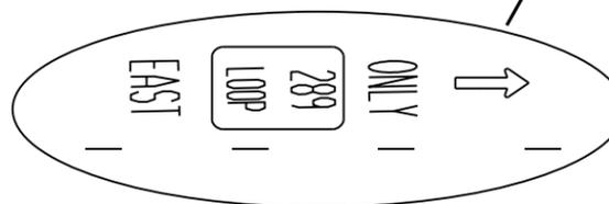
\* PAVEMENT MARKINGS MUST BE PLACED NEAR OR AT OVERHEAD SIGN AND FIELD VERIFIED BY INSPECTOR/ ENGINEER.
