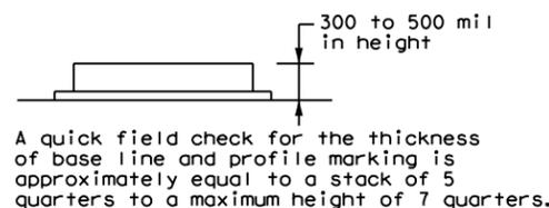
A quick field check for the thickness of base line and profile marking is approximately equal to a stack of 5 quarters to a maximum height of 7 quarters.
