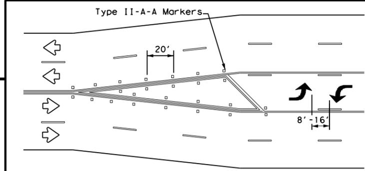
A two-way left-turn (TWLTL) lane-use arrow pavement marking should be used at or just downstream from the beginning of a two-way left-turn lane within a corridor. Repeating the marking after each intersection or dedicated turn bay is not required unless stated elsewhere in the plans.
