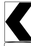
18" x 24" Sign (Maximum Sign Dimension) Chevron CWI-8, Opposing Traffic Lane Divider, Driveway Sign D10a, Keep Right R4 series or other signs as approved by Engineer
