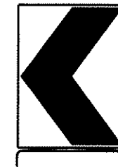
15' x 24" Sign (Maximum Sign Dimension) Chevron CW1-8, Opposing Traffic Lane Divider, Driveway sign D70s, Keep Right R4 series or other signs as approved by Engineer
