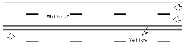
REFLECTORIZED PAVEMENT MARKINGS
