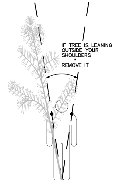
LEANING TREE REMOVAL
