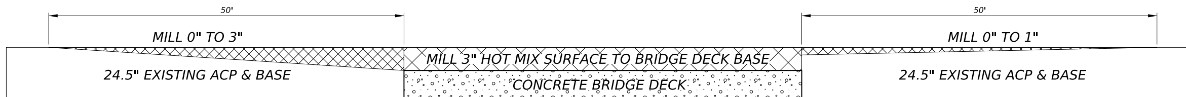
PROPOSED TIE-IN DETAIL: PHASE 1 DETAIL A-A MILL 0" TO 3" NOT TO SCALE
