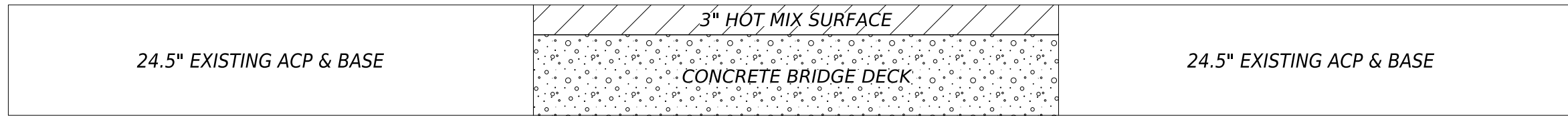
EXISTING TYPICAL SECTION
