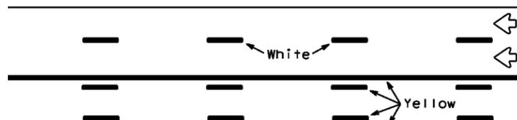
REFLECTORIZED PAVEMENT MARKINGS
