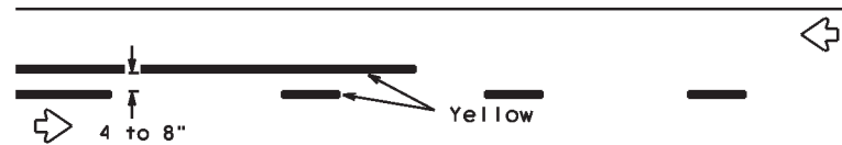
REFLECTORIZED PAVEMENT MARKINGS - PATTERN B
