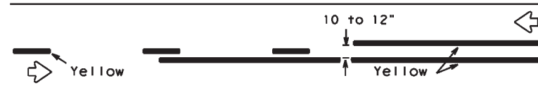
REFLECTORIZED PAVEMENT MARKINGS - PATTERN A
