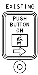
EXISTING R10-4b SIGN & PEDESTRIAN PUSH BUTTON W1, W2, W3, W4, W7 & W8 (TO REMAIN IN PLACE) W5 & W6 (SALVAGED, TO BE RE-USED)
