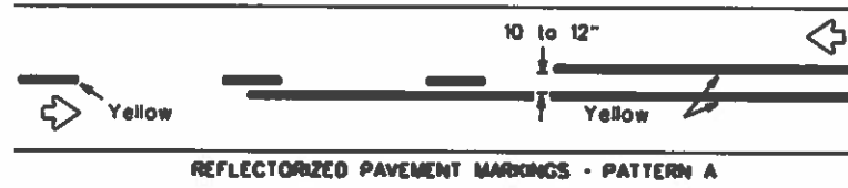
REFLECTORIZED PAVEMENT MARKINGS - PATTERN A
