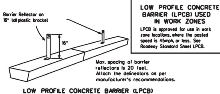
**LOW PROFILE CONCRETE BARRIER (LPCB) USED IN WORK ZONES**
