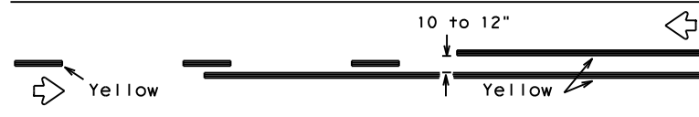
REFLECTORIZED PAVEMENT MARKINGS - PATTERN A
