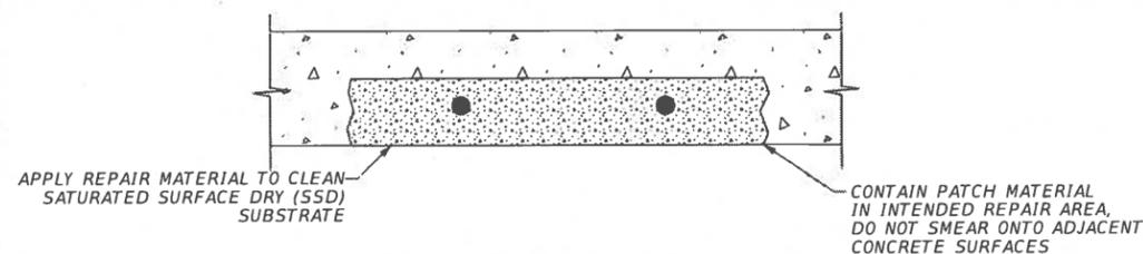
**STEP 3 - INTERMEDIATE SPALL REPAIR**
