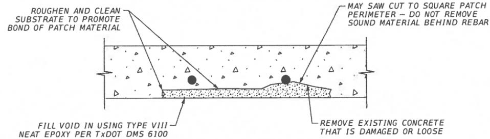
**STEP 2 - MINOR SPALL REPAIR**
