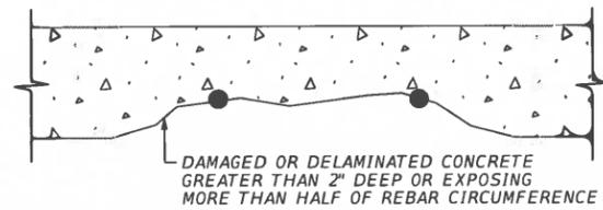
**STEP 1 - INTERMEDIATE SPALL REPAIR**
