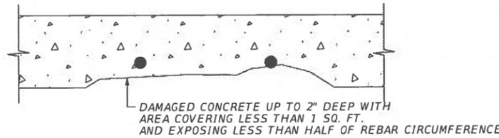
**STEP 1 - MINOR SPALL REPAIR**
