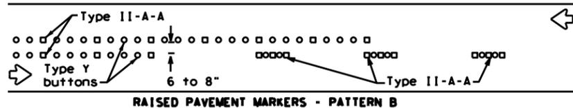
Pattern A is the TxDOT Standard, however Pattern B may be used if approved by the Engineer. Prefabricated markings may be substituted for reflectorized pavement markings.
