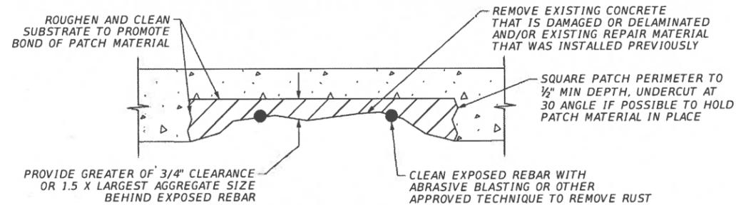
**STEP 2 - INTERMEDIATE SPALL REPAIR**
