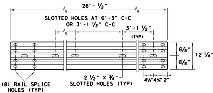
**ELEVATION 25'-0" (NOM.) W-BEAM SECTION**
