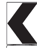
18" x 24" Sign (Maximum Sign Dimension) Chevron CWL-8, Opposing Traffic Lane Divider, Driveway sign D70a, Keep Right R4 series or other signs as approved by Engineer
