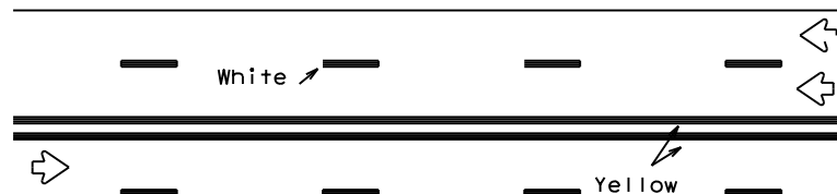
REFLECTORIZED PAVEMENT MARKINGS
