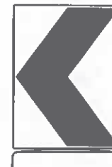
18" x 24" Sign (Maximum Sign Dimension) Chevron CWI-8, Opposing Traffic Lane Divider, Driveway sign D700, Keep Right R4 series or other signs as approved by Engineer
