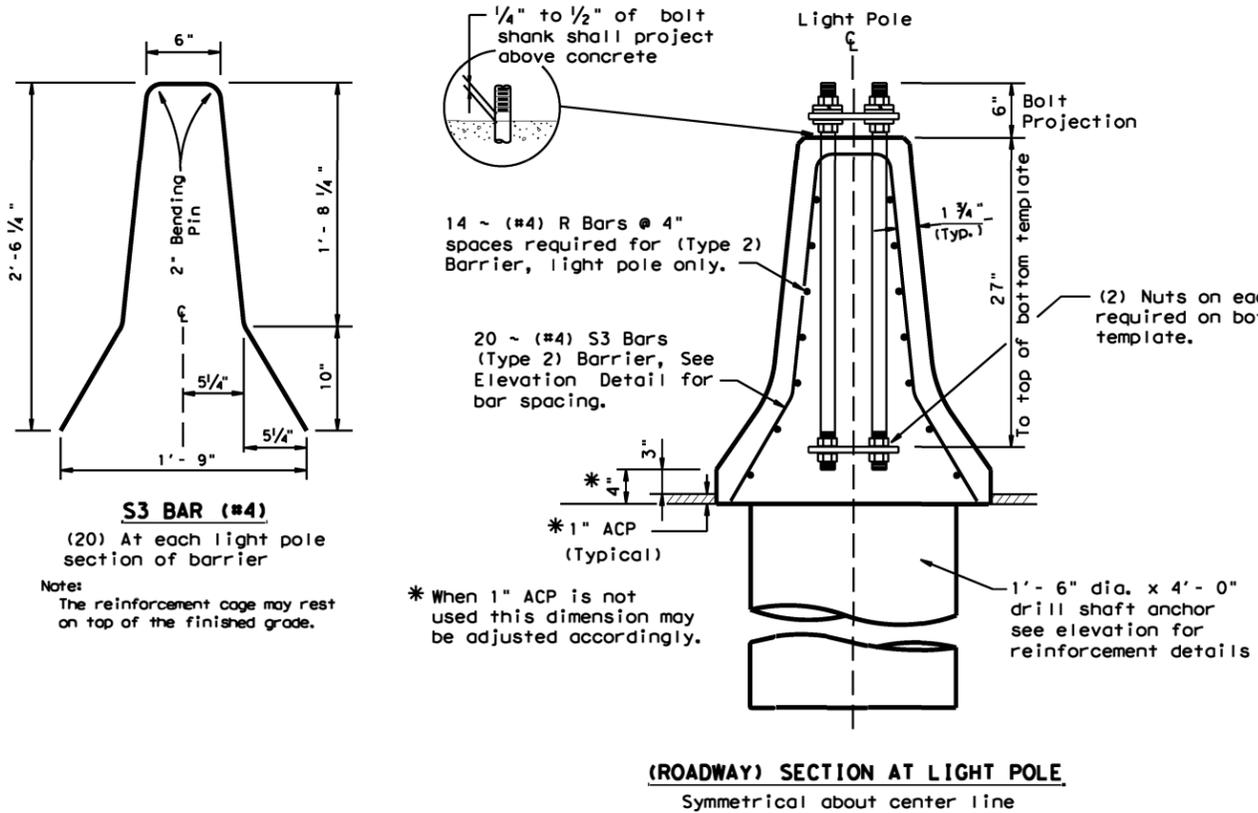
Schedule of reinforcement for each 10 foot cast-in-place section at light poles (excluding anchorage)
