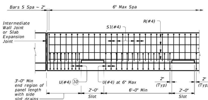
**OPTIONAL SIDE SLOT DRAIN DETAIL**
