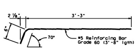
**DEFORMED BAR ANCHOR DETAILS**
