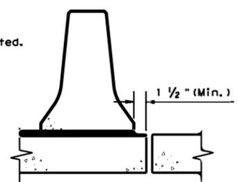
**Minimum Edge Distance From Longitudinal Joint**
