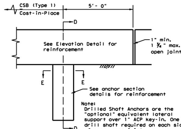
**DRILLED SHAFT ANCHOR
