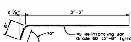
**DEFORMED BAR ANCHOR DETAILS**
