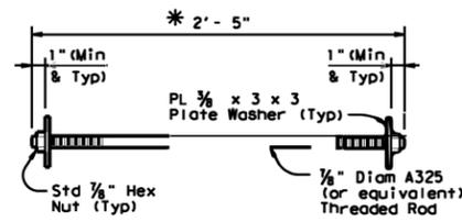
**CONNECTION BOLT OR THREADED ROD DETAIL**
