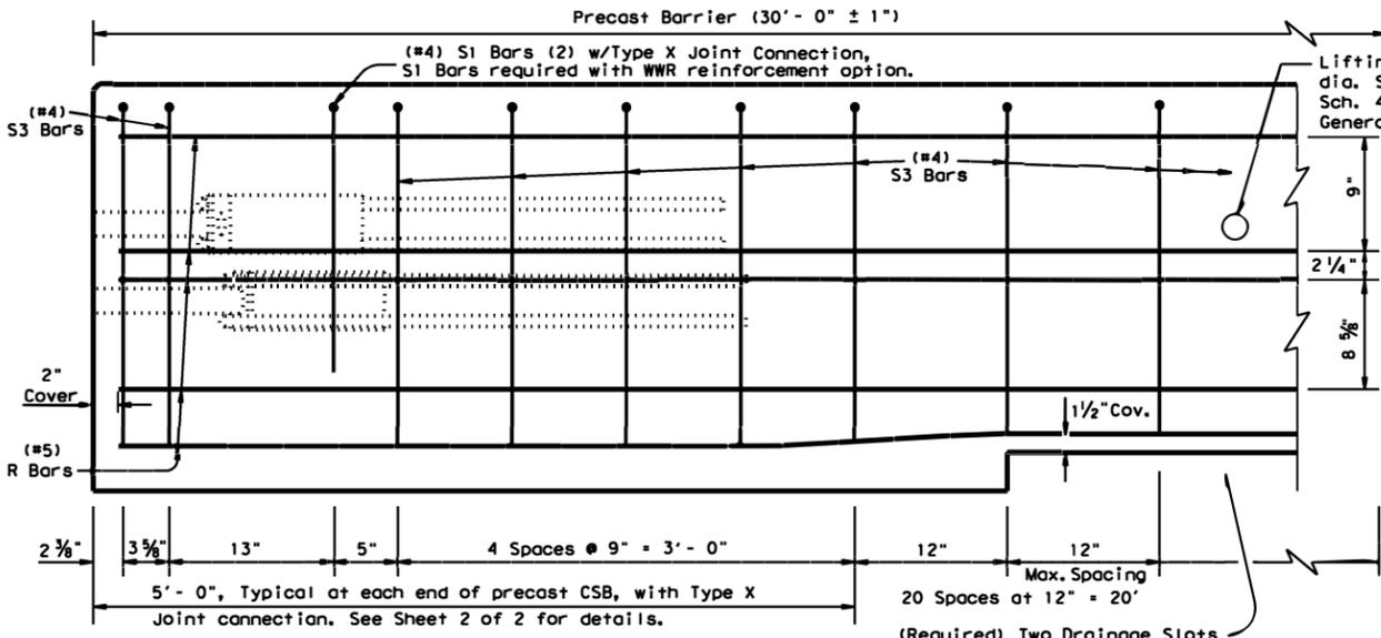
**Reinforcement for Precast (CSB) Concrete Safety Barrier (Type 1)**
