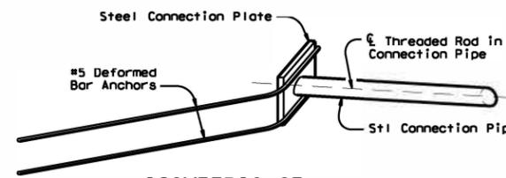
**ISOMETRIC OF TYPICAL WELDED ASSEMBLY**
