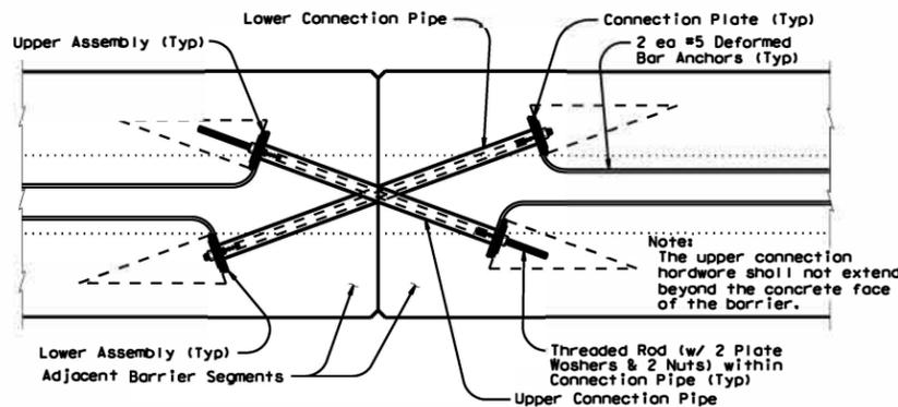
**TYPE X JOINT INSTALLATION DETAIL**
