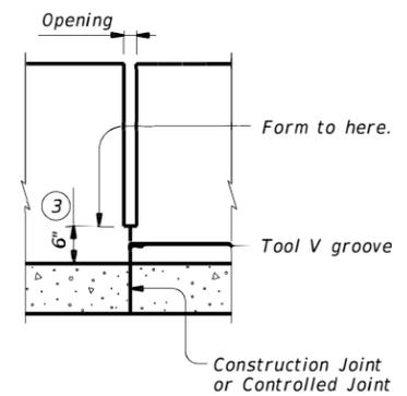
**INTERMEDIATE WALL JOINT DETAIL**
