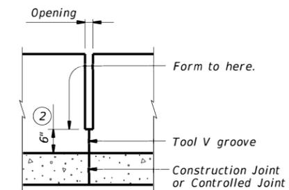
**INTERMEDIATE WALL JOINT DETAIL**
