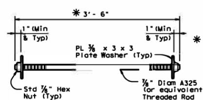
**CONNECTION BOLT OR THREADED ROD DETAIL**
