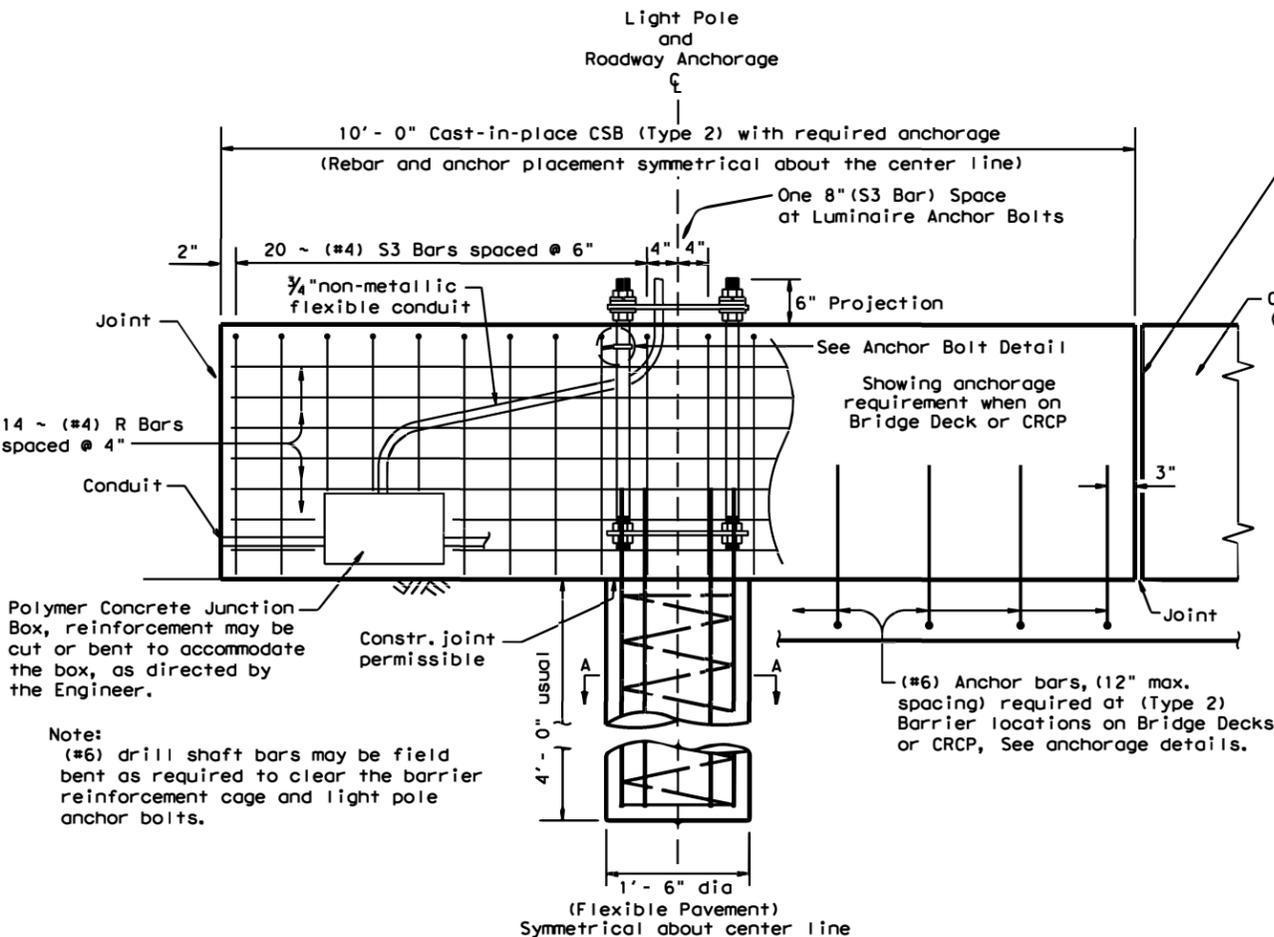
Each end of cast-in-place light pole section shall be formed to mate with the adjacent precast (Type 1) roadway barrier. The cast-in-place section shall be connected at each end to the precast sections in the same manner that precast sections are connected at joints as shown elsewhere.
