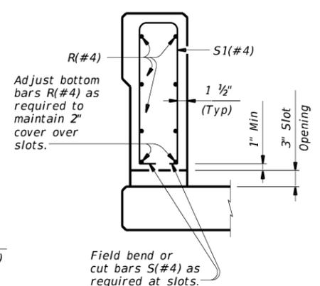
**SECTION THRU OPTIONAL SIDE SLOT DRAIN**
