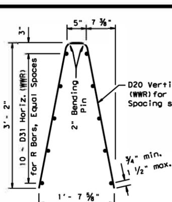
**Welded Wire Reinforcement (WWR) Option for Bars R and V1**
