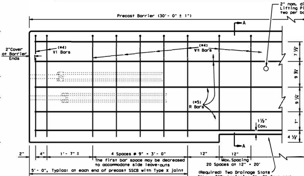
**Reinforcement for Precast (SSCB) Single Slope Concrete Barrier (Type 1)**
