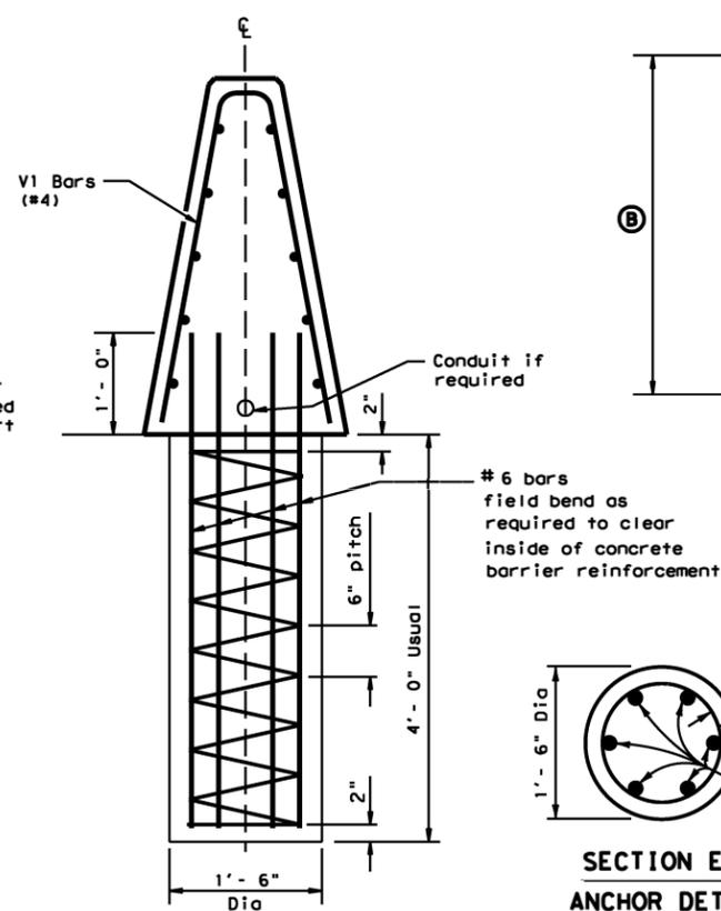
**SECTION D-D ANCHOR DETAIL**
