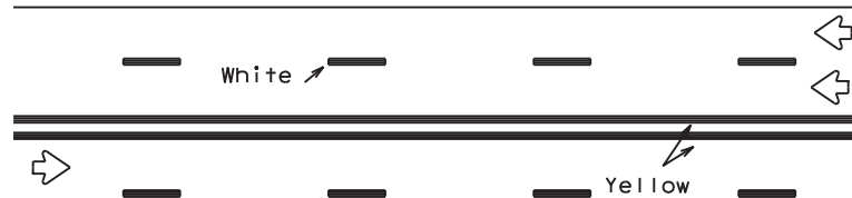
REFLECTORIZED PAVEMENT MARKINGS
