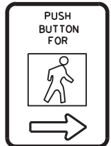
PEDESTRIAN PUSHBUTTON SIGN DETAILS
