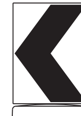
18" x 24" Sign (Maximum Sign Dimension) Chevron CW1-8, Opposing Traffic Lane Divider, Driveway sign D70a, Keep Right R4 series or other signs as approved by Engineer
