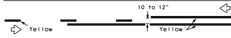
REFLECTORIZED PAVEMENT MARKINGS - PATTERN A
