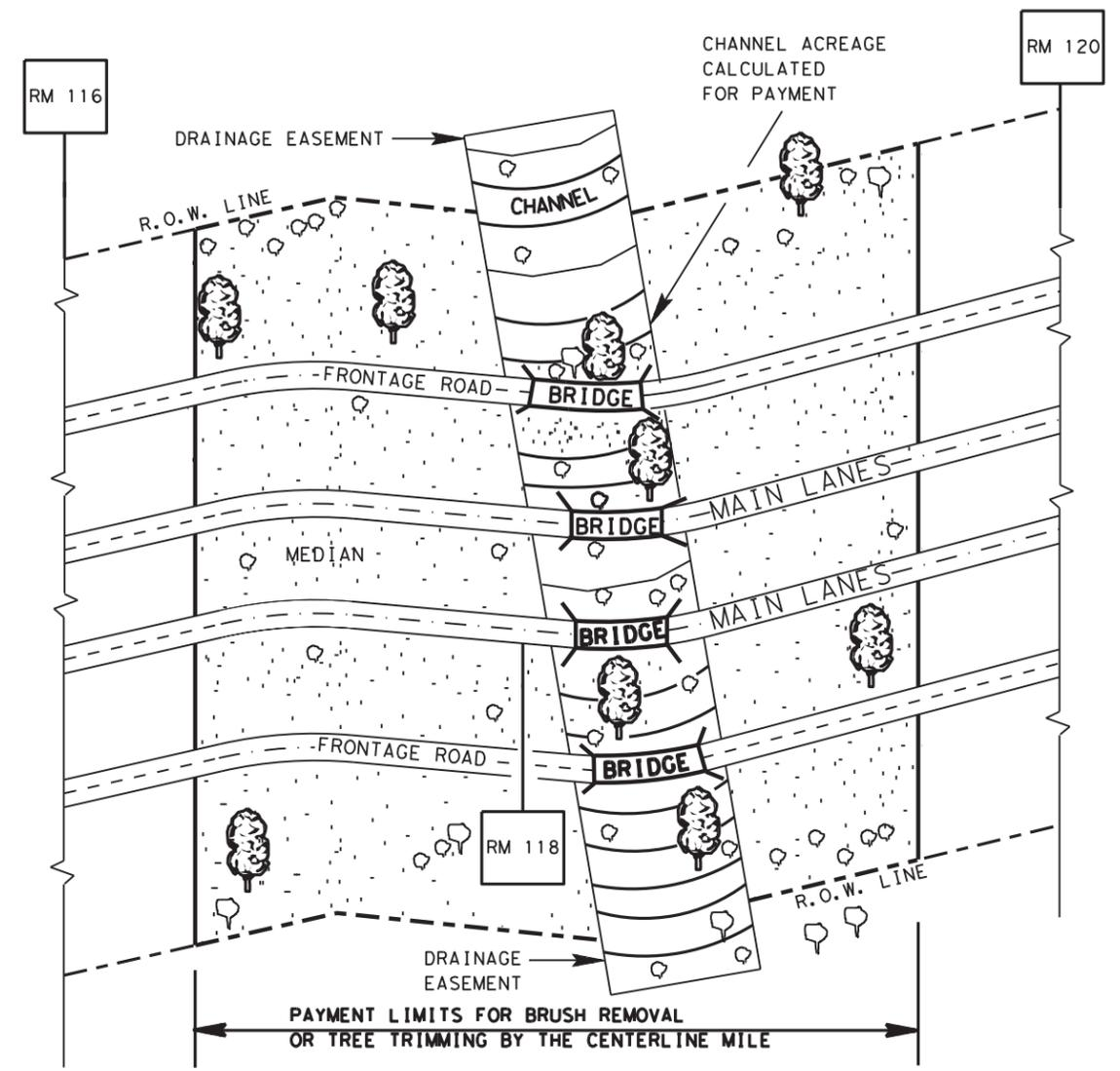
BRUSH REMOVED TO WITHIN 1" OF GROUND <4" DIAMETER TRUNK IS DEFINED AS BRUSH UNLESS OTHERWISE DIRECTED
