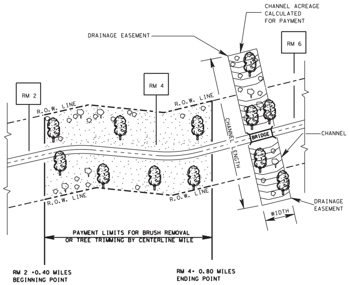
BRUSH REMOVED TO WITHIN 1" OF GROUND <4" DIAMETER TRUNK IS DEFINED AS BRUSH UNLESS OTHERWISE DIRECTED
