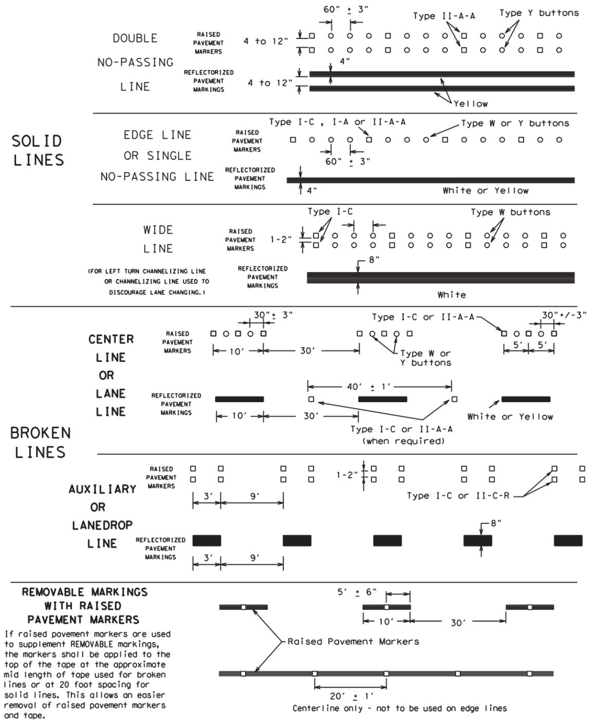
Raised pavement markers used as standard pavement markings shall be from the approved products list and meet the requirements of Item 672 "RAISED PAVEMENT MARKERS."
