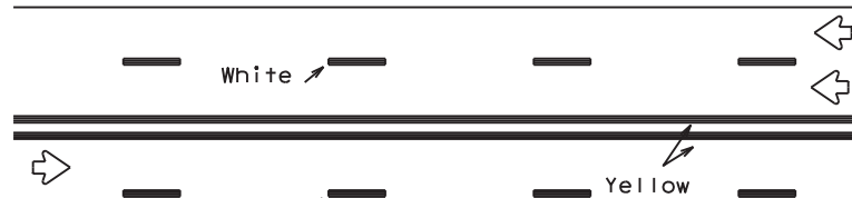
REFLECTORIZED PAVEMENT MARKINGS
