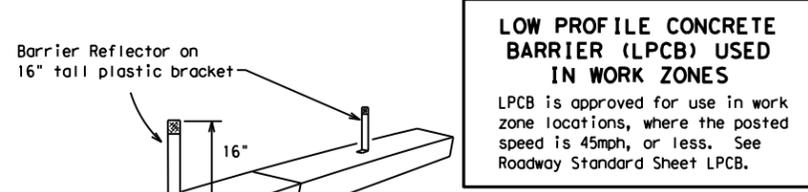
**LOW PROFILE CONCRETE BARRIER (LPCB) USED IN WORK ZONES**
