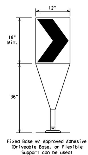
1. The chevron shall be a vertical rectangle with a minimum size of 12 by 18 inches.
