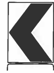
18" x 24" Sign (Maximum Sign Dimension) Chevron CW1-8, Opposing Traffic Lane Divider, Driveway sign D70a, Keep Right R4 series or other signs as approved by Engineer
