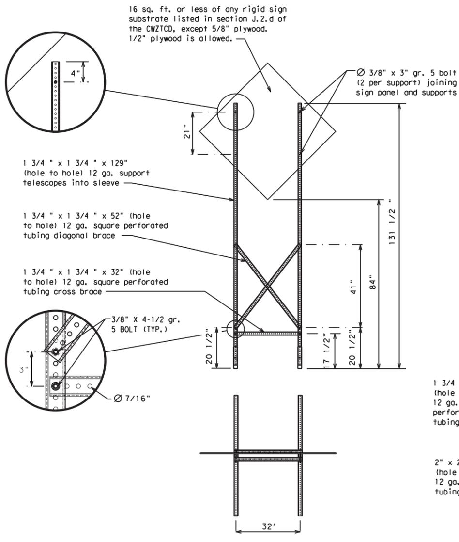
16 sq. ft. or less of any rigid sign substrate listed in section J.2.d of the CWZTCD, except 5/8\"/>
