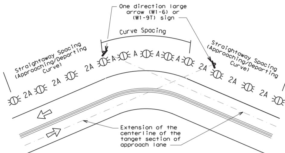
Curves less than 1 degree do not normally require delineators.
