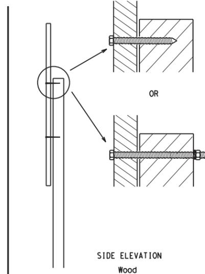
Attachment to wooden supports will be by bolts and nuts or screws. Use TxDOT's or manufacturer's recommended procedures for attaching sign substrates to other types of sign supports
