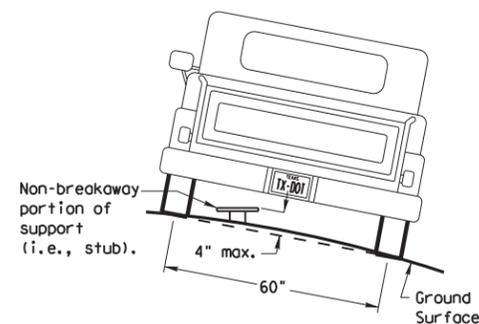
To avoid vehicle undercarriage snagging, any substantial remains of a breakaway support, when it is broken away, should not project more than 4 inches above a 60-inch chord (i.e., typical space between wheel paths).
