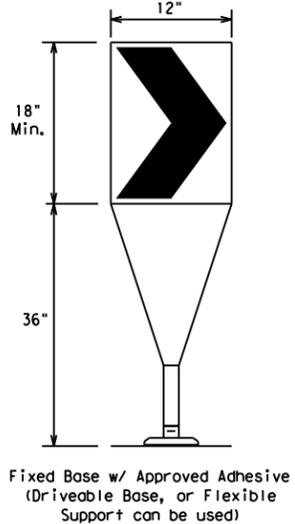
Fixed Base w/ Approved Adhesive (Driveable Base, or Flexible Support can be used)
