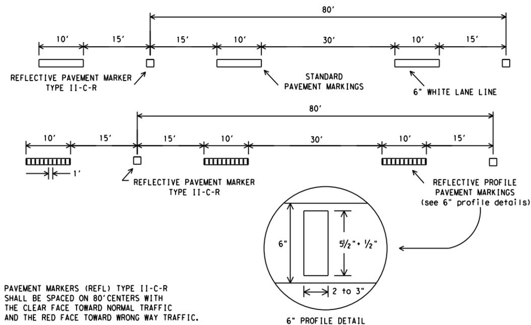
PAVEMENT MARKERS (REFL) TYPE II-C-R SHALL BE SPACED ON 80' CENTERS WITH THE CLEAR FACE TOWARD NORMAL TRAFFIC AND THE RED FACE TOWARD WRONG WAY TRAFFIC.
