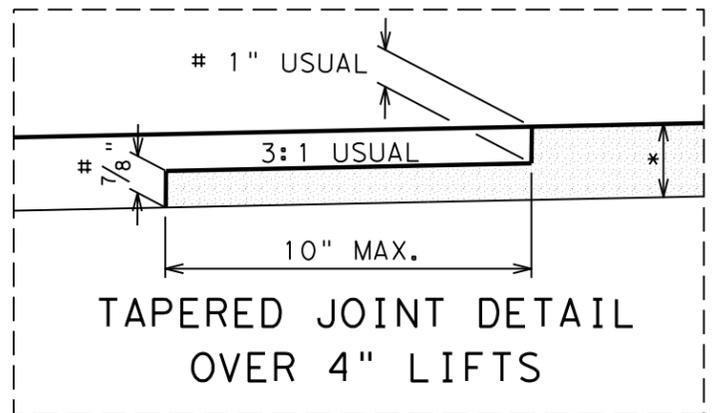
@ IF BACKFILLED SLOPE IS LESS THAN 3:1, COVER WEDGE WITH APPROVED BACKFILL.
