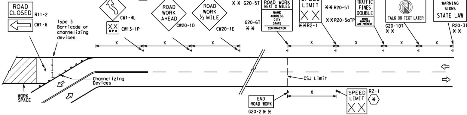
**SAMPLE LAYOUT OF SIGNING FOR WORK BEGINNING AT THE CSJ LIMITS**
