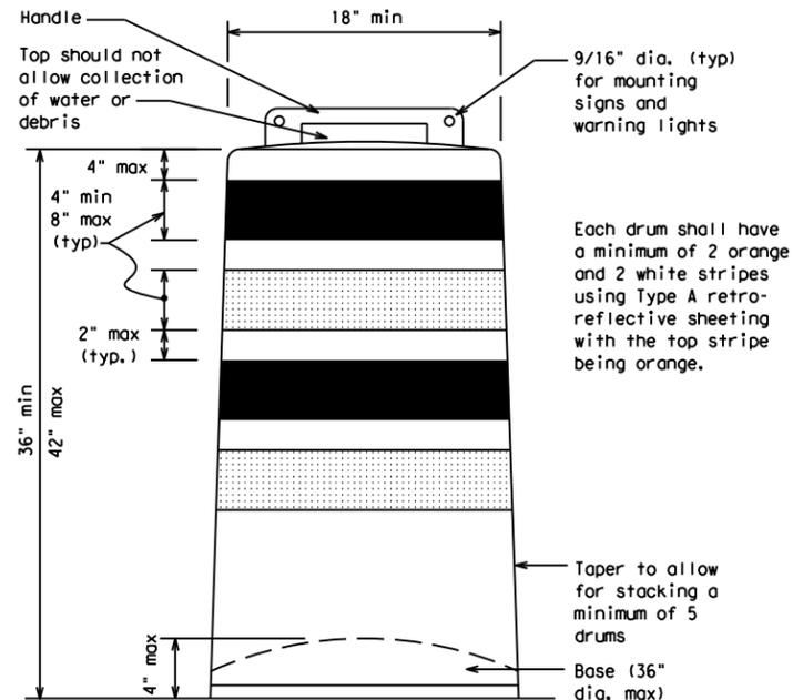
Each drum shall have a minimum of 2 orange and 2 white stripes using Type A retro-reflective sheeting with the top stripe being orange.
