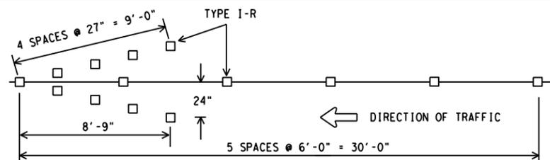
ALL RAISED MARKERS IN THE WRONG WAY ARROW SHALL BE TYPE I-R REFLECTORIZED PAVEMENT MARKERS WITH THE REFLECTORIZED SURFACE FACING THE WRONG WAY TRAFFIC. TYPE II-C-R SHALL NOT BE USED. REFLECTORIZED WRONG WAY ARROWS, NOT TO EXCEED TWO, MAY BE PLACED ON EXIT RAMP. LOCATION OF THE ARROWS SHALL BE AS SHOWN IN THE PLANS OR AS DIRECTED BY THE ENGINEER.
