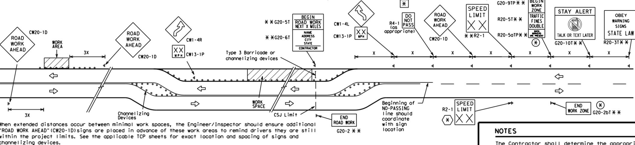
When extended distances occur between minimal work spaces, the Engineer/Inspector should ensure additional "ROAD WORK AHEAD" (CW20-1D) signs are placed in advance of these work areas to remind drivers they are still within the project limits. See the applicable TCP sheets for exact location and spacing of signs and channelizing devices.
