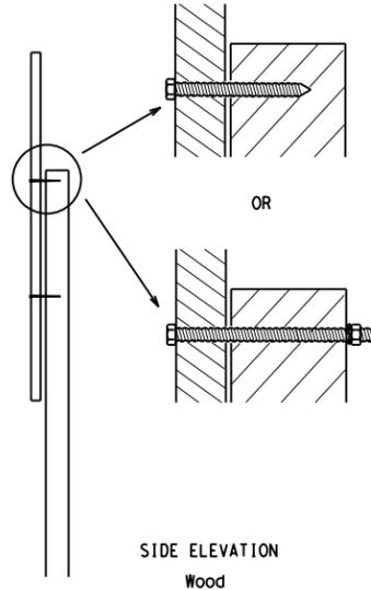
**Nails shall NOT be allowed. Each sign shall be attached directly to the sign support. Multiple signs shall not be joined or spliced by any means. Wood supports shall not be extended or repaired by splicing or other means.**
