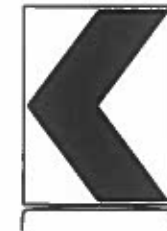
18" x 24" Sign (Maximum Sign Dimension) Chevron CWI-8, Opposing Traffic Lane Divider, Driveway sign 070a, Keep Right R4 series or other signs as approved by Engineer
