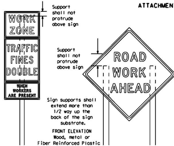
Splicing embedded perforated square metal tubing in order to extend post height will only be allowed when the splice is made using four bolts, two above and two below the splice point. Splice must be located entirely behind the sign substrate, not near the base of the support. Splice insert lengths should be at least 5 times nominal post size, centered on the splice and of at least the same gauge material.
