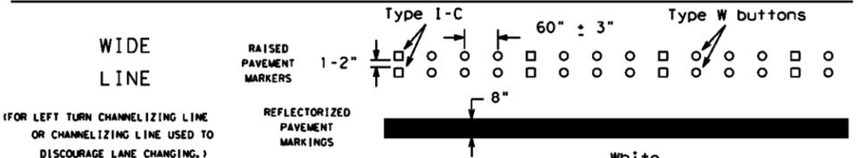
(FOR LEFT TURN CHANNELIZING LINE OR CHANNELIZING LINE USED TO DISCOURAGE LANE CHANGING.)
