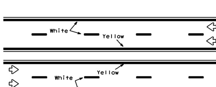
REFLECTORIZED PAVEMENT MARKINGS
