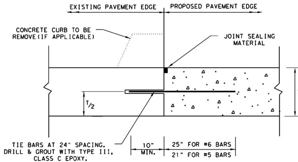
1. BEFORE WIDENING WORK, DEMONSTRATE THAT THE BOND STRENGTH OF THE EPOXY-GROUTED TIE BARS MEETS THE REQUIREMENTS OF PULL-OUT TEST SPECIFIED IN ITEM 361.
