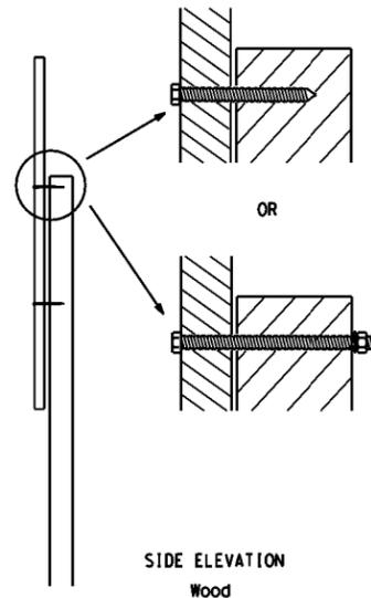
**Nails shall NOT be allowed. Each sign shall be attached directly to the sign support. Multiple signs shall not be joined or spliced by any means. Wood supports shall not be extended or repaired by splicing or other means.**
