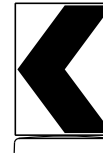
18" x 24" Sign (Maximum Sign Dimension) Chevron CW1-8, Opposing Traffic Lane Divider, Driveway Sign D70a, Keep Right R4 series or other signs as approved by Engineer
