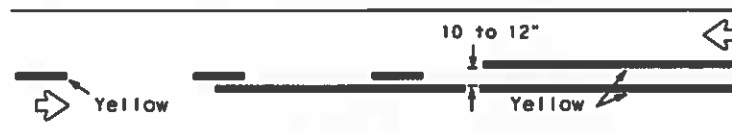
REFLECTORIZED PAVEMENT MARKINGS - PATTERN A
