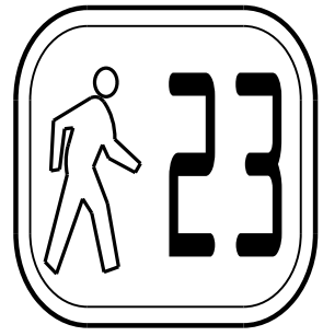
PEDESTRIAN HEAD (ONE-SECTION HEAD DISPLAYS WALK AND DON'T WALK SYMBOLS AND COUNTDOWN MODULE)
