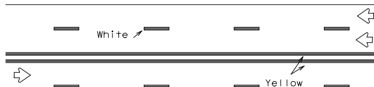
REFLECTORIZED PAVEMENT MARKINGS
