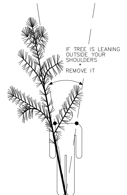
LEANING TREE REMOVAL
