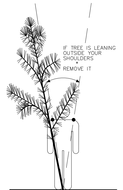
LEANING TREE REMOVAL
