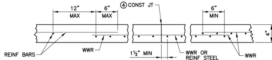
**CONCRETE RIPRAP REINFORCEMENT DETAILS** ③
