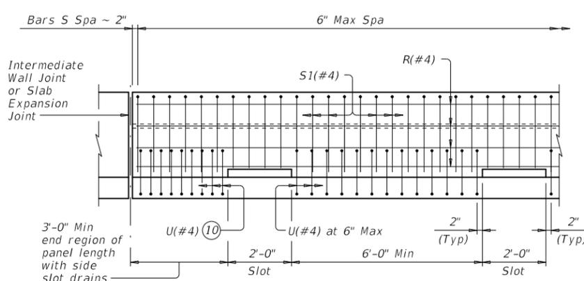
OPTIONAL SIDE SLOT DRAIN DETAIL
