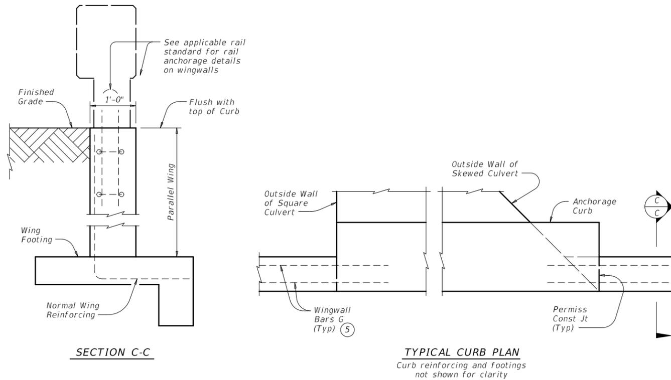
**INSTALLATION AT PARALLEL CULVERT WINGWALLS**
