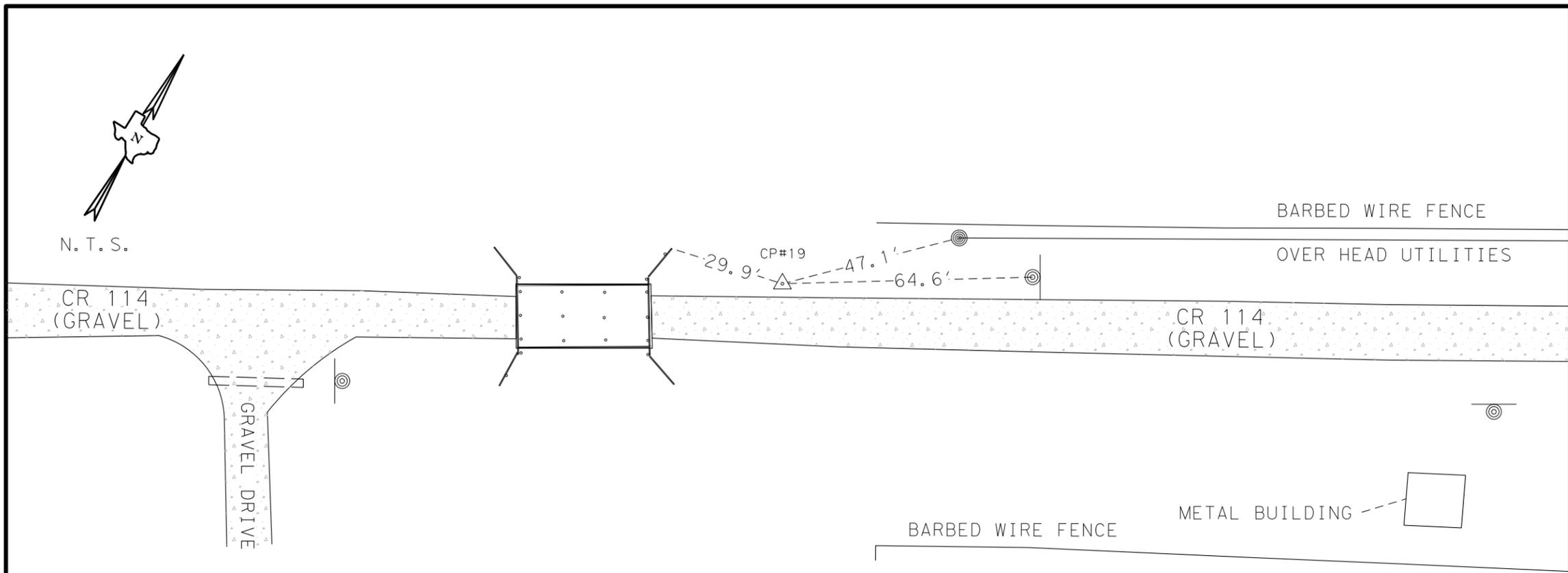
CP# 19 IS A 5/8-INCH IRON ROD WITH RED PLASTIC CAP STAMPED "CP&Y TRAV. POINT" LOCATED IN WHARTON COUNTY, TX., LOCATED ON THE NORTH SIDE OF CR 114, +/- 29.9' EAST OF A WINGWALL LOCATED AT THE NORTHWEST CORNER OF A BRIDGE ON CR 114, +/- 47.1' SOUTHWEST OF A POWERPOLE LOCATED ON THE NORTH SIDE OF CR 114, AND +/- 64.6' SOUTHWEST OF A WEIGHT LIMIT SIGN LOCATED ON THE NORTH SIDE OF CR 114.
