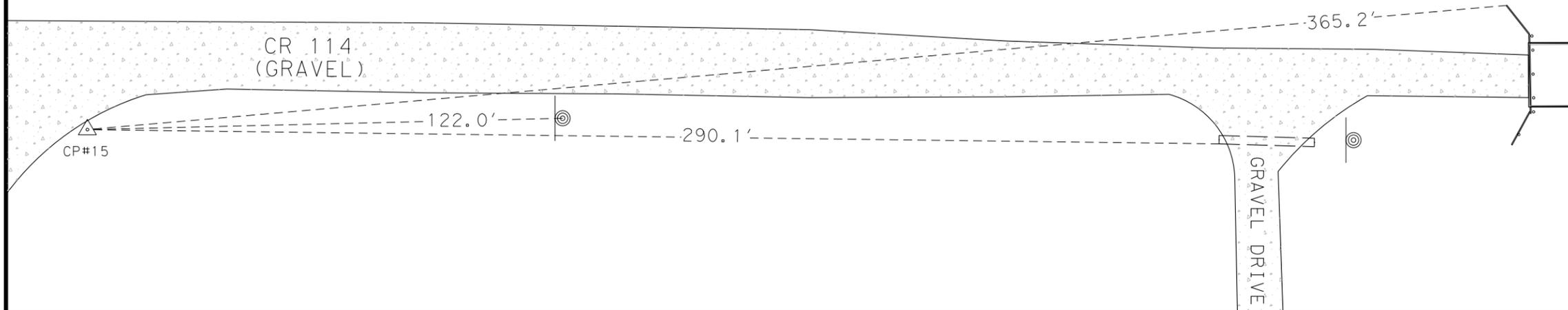
CP# 15 IS A 5/8-INCH IRON ROD WITH RED PLASTIC CAP STAMPED "CP&Y TRAV. POINT" LOCATED IN WHARTON COUNTY, TX., LOCATED ON THE SOUTH SIDE OF CR 114, +/- 365.2' SOUTHWEST OF A WINGWALL LOCATED AT THE SOUTHWEST CORNER OF A BRIDGE ON CR 114, +/- 290.1' SOUTHWEST OF A CRUSHED CMP LOACTED ON THE SOUTH SIDE OF CR 114, AND +/- 122.0' SOUTHWEST OF A SPEED LIMIT SIGN LOCATED ON THE SOUTH SIDE OF CR 114.
