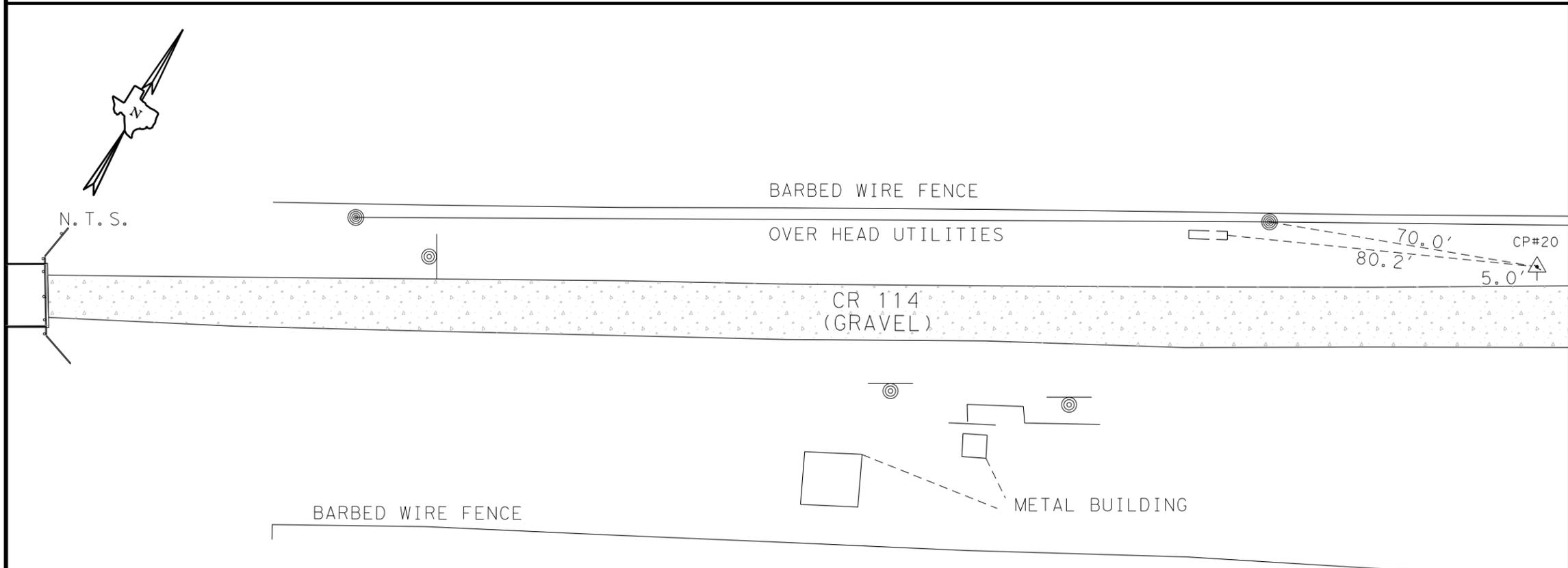
CP# 20 IS A 5/8-INCH IRON ROD WITH RED PLASTIC CAP STAMPED "CP&Y TRAV. POINT" LOCATED IN WHARTON COUNTY, TX., LOCATED ON THE NORTH SIDE OF CR 114, +/- 80.2' NORTHEAST OF A 12" CMP LOCATED ON THE NORTH SIDE OF CR 114, +/- 70.0' NORTHEAST OF A POWERPOLE LOCATED ON THE NORTH SIDE OF CR 114, AND +/- 5.0' NORTHWEST OF THE NORTH EDGE OF PAVEMENT OF CR 114.
