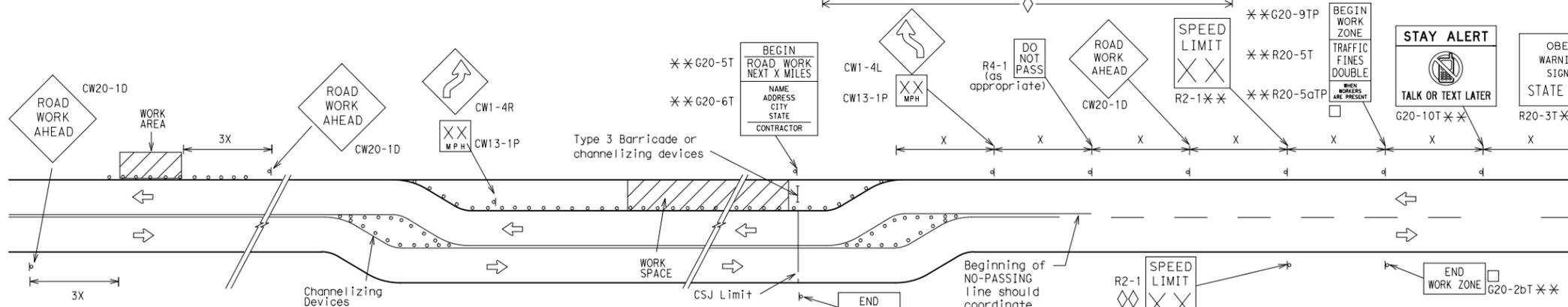
When extended distances occur between minimal work spaces, the Engineer/Inspector should ensure additional "ROAD WORK AHEAD" (CW20-1D) signs are placed in advance of these work areas to remind drivers they are still within the project limits. See the applicable TCP sheets for exact location and spacing of signs and channelizing devices.
