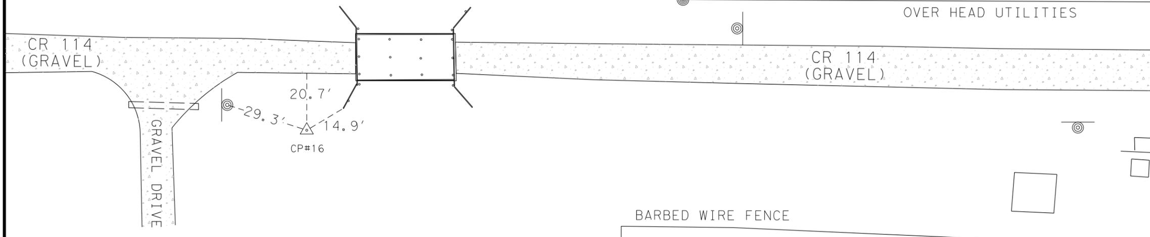
CP# 16 IS A 5/8-INCH IRON ROD WITH RED PLASTIC CAP STAMPED "CP&Y TRAV. POINT" LOCATED IN WHARTON COUNTY, TX., LOCATED ON THE SOUTH SIDE OF CR 114, +/- 14.9' SOUTHWEST OF A WINGWALL LOCATED AT THE SOUTHEAST CORNER OF A BRIDGE LOCATED ON CR 114, +/- 20.7' SOUTH EAST OF THE SOUTH EDGE OF PAVEMENT FOR CR 114, AND +/- 29.3' EAST OF A WEIGHT LIMIT SIGN LOCATED ON THE SOUTH SIDE OF CR 114.
