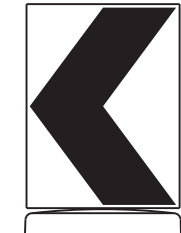
18" x 24" Sign (Maximum Sign Dimension) Chevron CW1-8, Opposing Traffic Lane Divider, Driveway sign D70a, Keep Right R4 series or other signs as approved by Engineer
