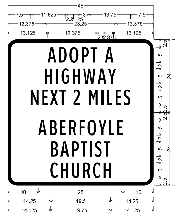
D14-4T-2_48x48; 3.000" Radius, 1.000" Border, White on Blue; "ADOPT A", ClearviewHwy-1-W; "HIGHWAY", ClearviewHwy-1-W; "NEXT 2 MILES", ClearviewHwy-1-W; 3.000" Radius, 1.000" Border, White on Blue; "ABERFOYLE", ClearviewHwy-1-W; "BAPTIST", ClearviewHwy-1-W; "CHURCH", ClearviewHwy-1-W;
