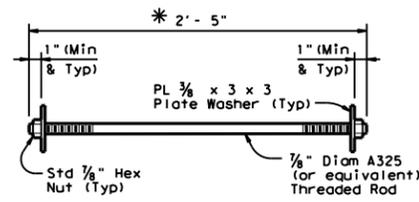
**CONNECTION BOLT OR THREADED ROD DETAIL**
