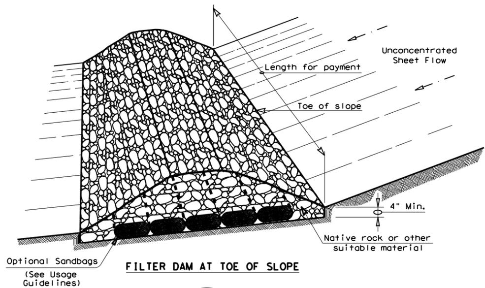
**FILTER DAM AT TOE OF SLOPE**
