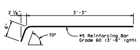
**DEFORMED BAR ANCHOR DETAILS**
