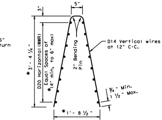
**Welded Wire Reinforcement (WWR) Option for Bars V1 and H1**
