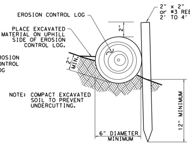
**STAKE AND LASHING ANCHORING DETAIL**
