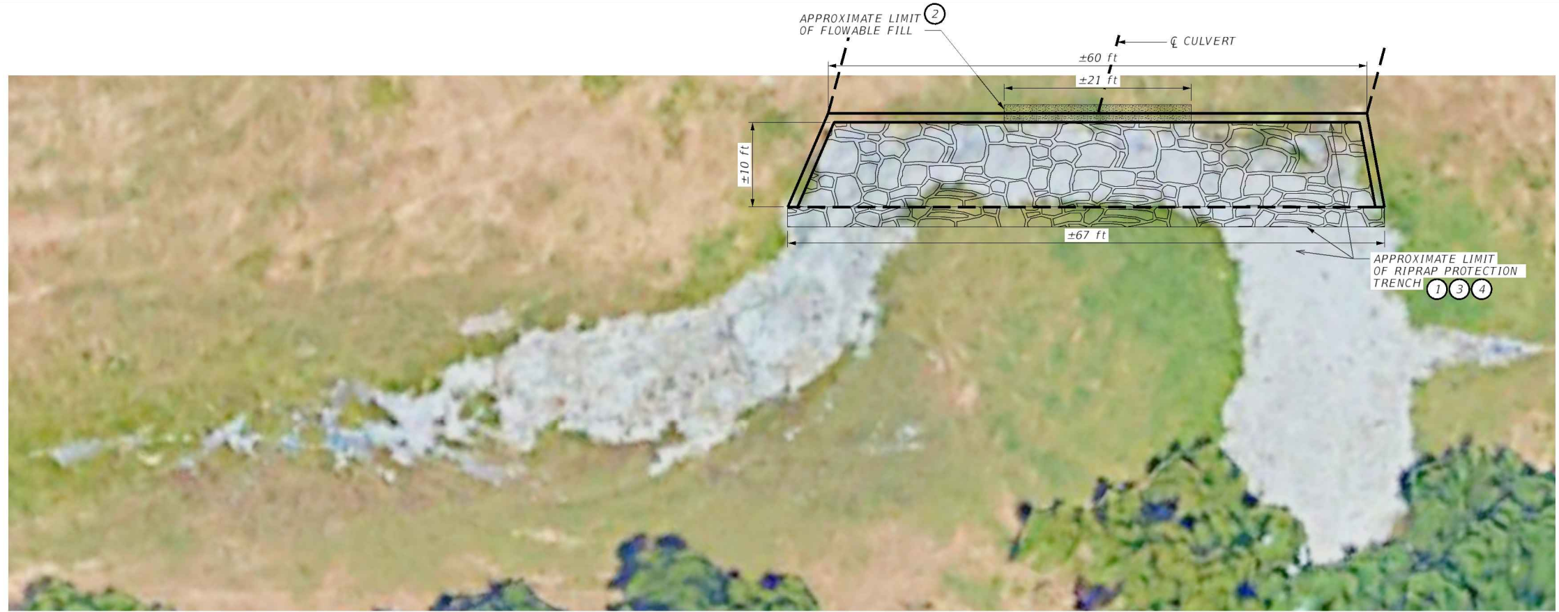
PLAN - CULVERT SOUTH END RIPRAP ①
