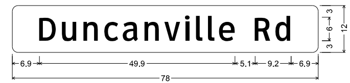
D3-1G(1) 6in; 1.5" Radius, No border, White on Green; "Duncanville Rd", ClearviewHwy-3-W; SHEET 15 SIGN 1 SHEET 15 SIGN 7
