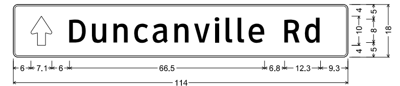
D1-1 8in UP; 1.5" Radius, 0.5" Border, White on Green; Standard Arrow Custom 10.0" X 7.1" 90"; "Duncanville Rd", ClearviewHwy-3-W;
