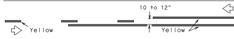
REFLECTORIZED PAVEMENT MARKINGS - PATTERN A
