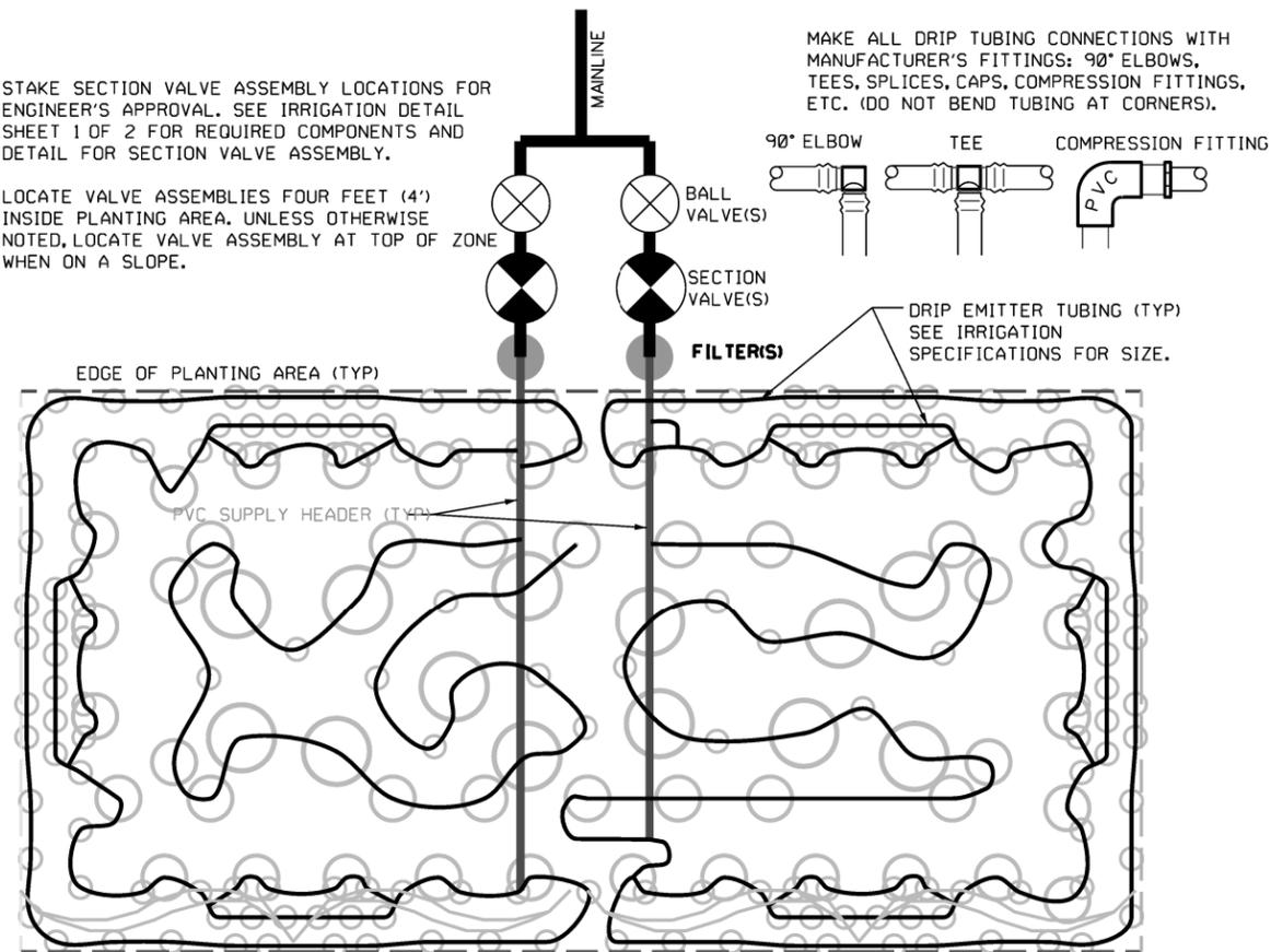
DRIP EMITTER TUBING SECTION (TYP) SHALL BE APPROX. EQUAL TO OTHER SECTION SIZES.
