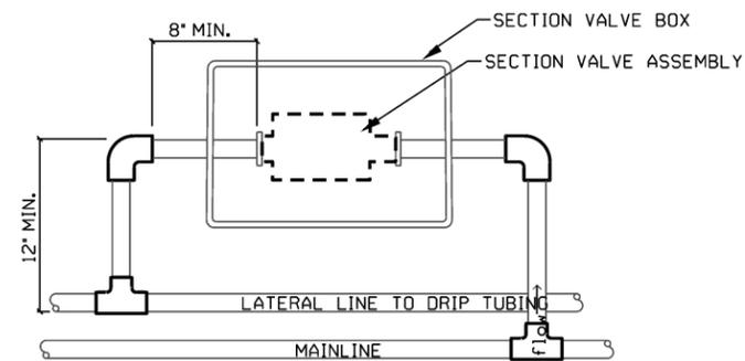
**PLAN OF PIPING TO SECTION VALVE ASSEMBLY**
