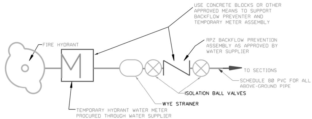
**TYPICAL TEMPORARY METER ASSEMBLY (PLAN)**
