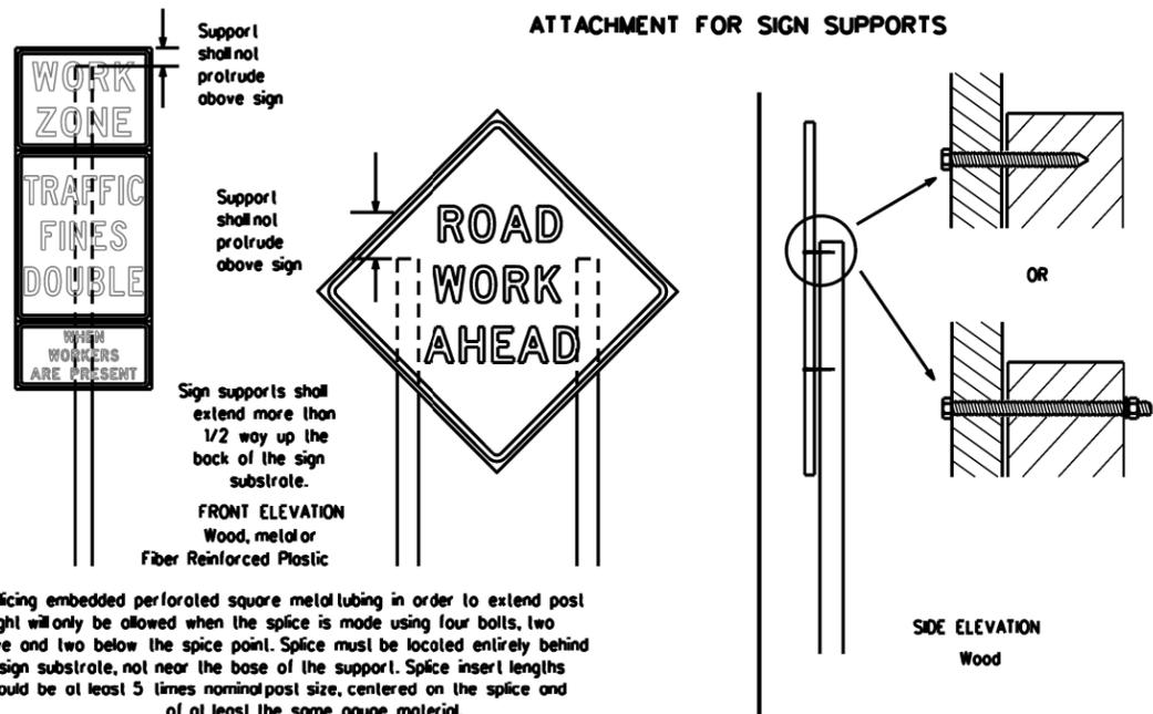
Attachment to wooden supports will be by bolts and nuts or screws. Use TxDOT's or manufacturer's recommended procedures for attaching sign substrates to other types of sign supports
