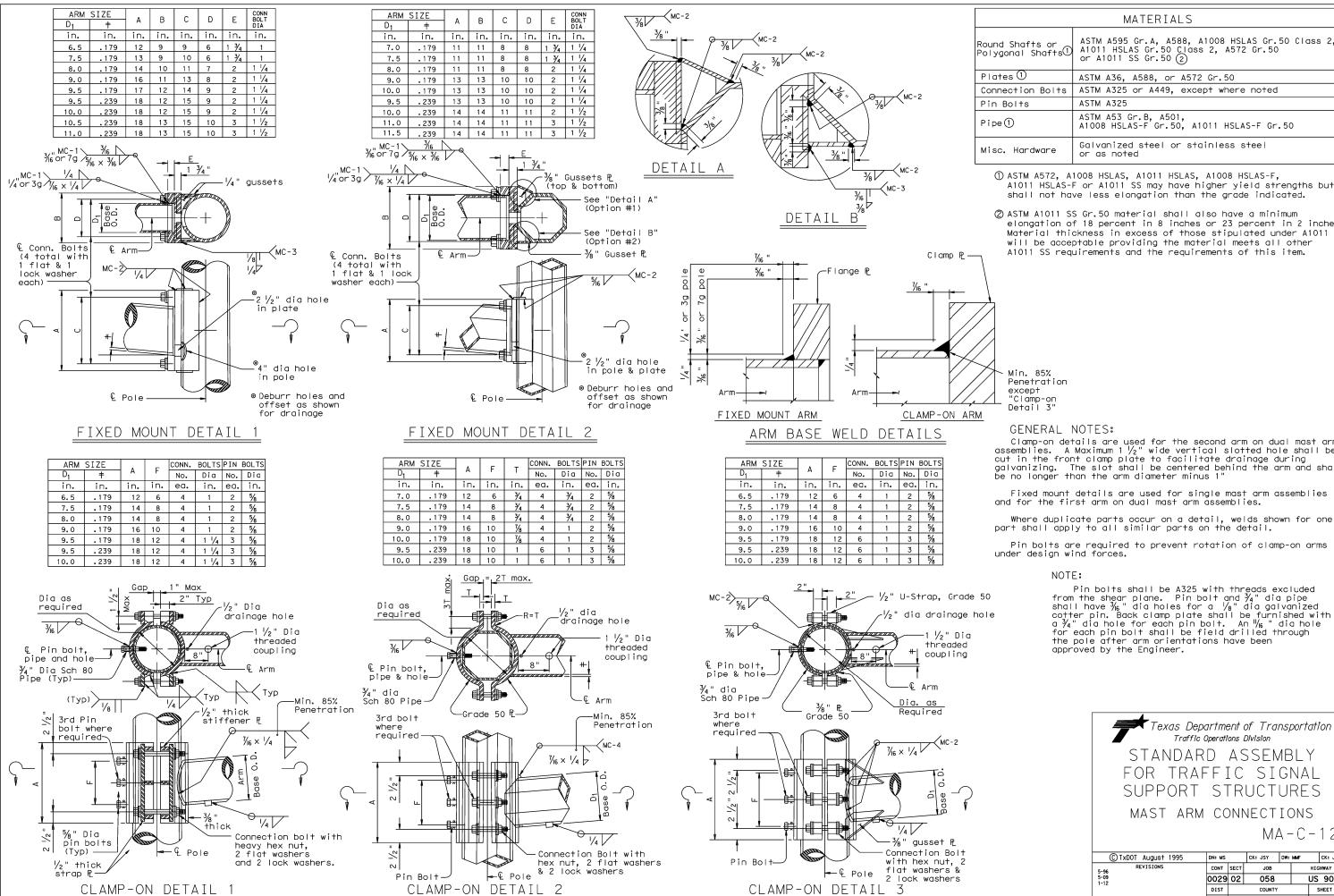
ASTM A595 Gr.A, A588, A1008 HSLAS Gr.50 Class 2, A1011 HSLAS Gr.50 Class 2, A572 Gr.50 or A1011 SS Gr.50 (2) ASTM A325 or A449, except where noted ASTM A53 Gr.B, A501, A1008 HSLAS-F Gr.50, A1011 HSLAS-F Gr.50 Galvanized steel or stainless stee or as noted
