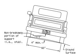
To avoid vehicle undercarriage snagging, any substantial remains of a breakaway support, when it is broken away, should not project more than 4 inches above a 60-inch chord (i.e., typical space between wheel paths).
