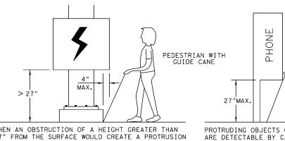
WHEN AN OBSTRUCTION OF A HEIGHT GREATER THAN 27" FROM THE SURFACE WOULD CREATE A PROTRUSION OF MORE THAN 4" INTO THE PEDESTRIAN CIRCULATION AREA, CONSTRUCT ADDITIONAL CURB OR FOUNDATION AT THE BOTTOM TO PROVIDE A MAXIMUM 4" OVERHANG.
