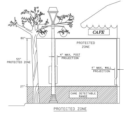
NOTE: IN PEDESTRIAN CIRCULATION AREA, MAXIMUM 4" PROJECTION FOR POST OR WALL MOUNTED OBJECTS BETWEEN 27" AND 80" ABOVE THE SURFACE.
