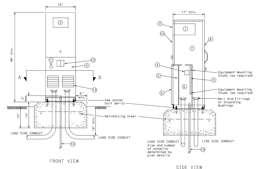
TYPE C shown, TYPE A similar except that TYPE A shall have individual circuit breakers (CB) mounted on an equipment mounting
