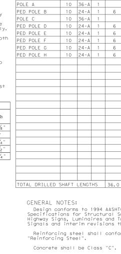
Design conforms to 1994 AASHTO Standard Specifications for Structural Supports for Highway Signs, Luminaires and Traffic Signals and interim revisions thereto.
