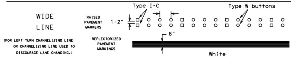
(FOR LEFT TURN CHANNELIZING LINE OR CHANNELIZING LINE USED TO DISCOURAGE LANE CHANGING.)
