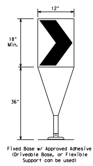
1. The chevron shall be a vertical rectangle with a minimum size of 12 by 18 inches.
