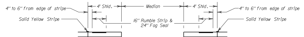
Milled Rumble Strip Detail Use Option 4 shown on RS(1)-13.
