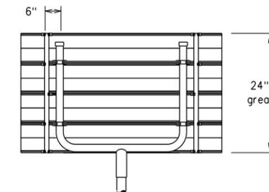
Use Extruded Alum. Windbeam as stiffeners
