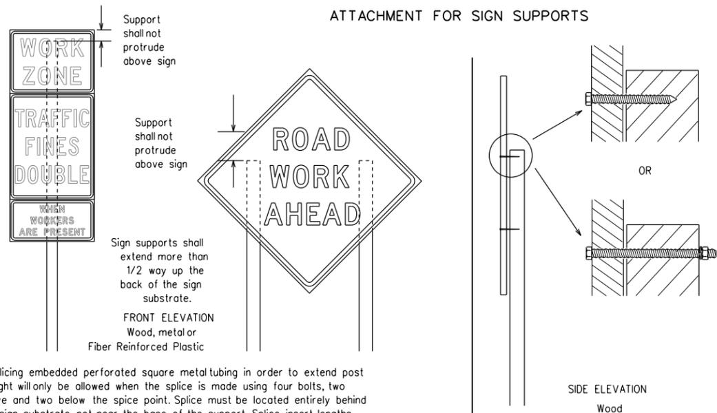
Attachment to wooden supports will be by bolts and nuts or screws. Use TxDOT's or manufacturer's recommended procedures for attaching sign substrates to other types of sign supports
