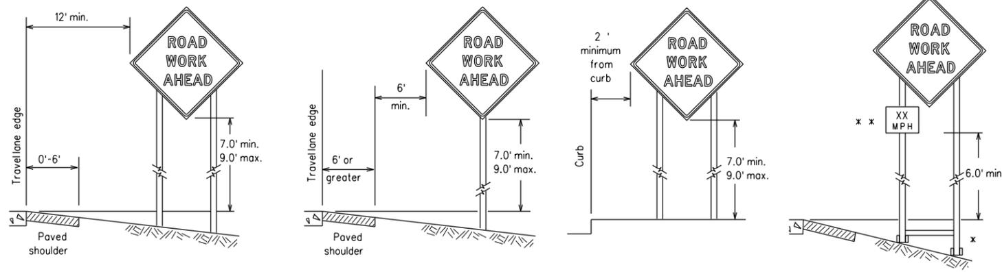
\* When placing skid supports on unlevel ground, the leg post lengths must be adjusted so the sign appears straight and plumb. Objects shall NOT be placed under skids as a means of leveling.
