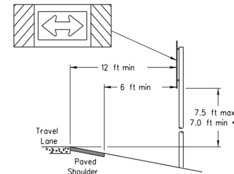
When this sign is needed at the end of a two-lane, two way roadway, the right edge of the sign should be in line with the centerline of the roadway. Place as close to ROW as practical.
