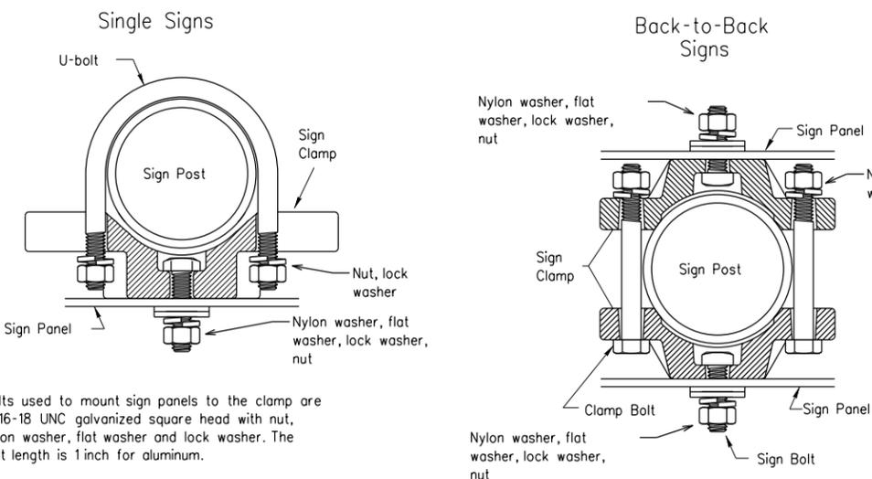
Bolts used to mount sign panels to the clamp are 5/16-18 UNC galvanized square head with nut, nylon washer, flat washer and lock washer. The bolt length is 1 inch for aluminum.
