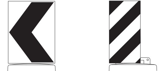
18" x 24" Sign (Maximum Sign Dimension) Chevron CWI-8, Opposing Traffic Lane Divider, Driveway sign D70a, Keep Right R4 series or other signs as approved by Engineer 12" x 24" Vertical Panel mount with diagonals sloping down towards travel way
