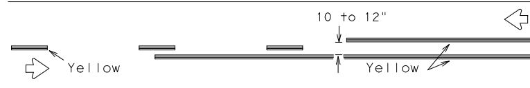
REFLECTORIZED PAVEMENT MARKINGS - PATTERN A
