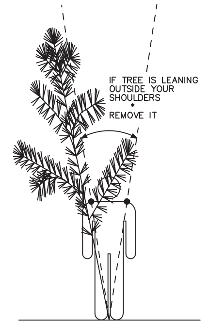
LEANING TREE REMOVAL
