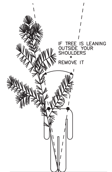
LEANING TREE REMOVAL
